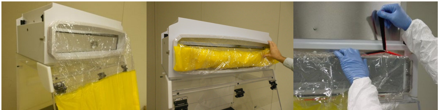
Install the filter bag | Roll bag up into flange | Secure with strap
