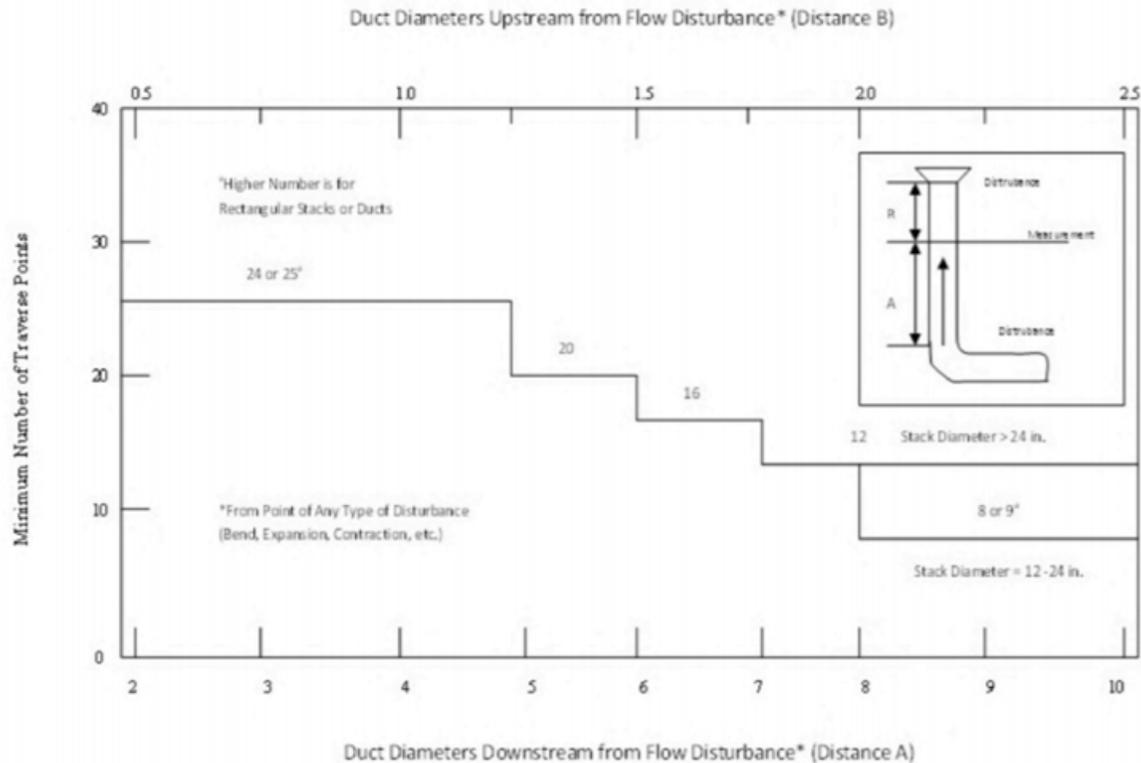
Figure 1-3. Minimum number of traverse points for an isokinetic sampling
