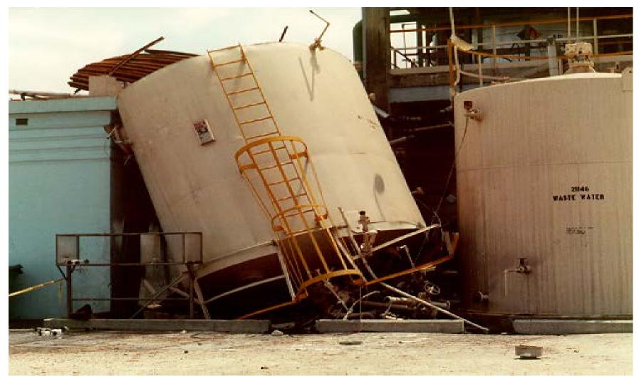
1988: Organic layer floating on water in tank. Tank draining to sewer trench. Welding overhead. Tank emptied. Welding spark to trench. Flashback into tank. Tank launched and turned upside down.
