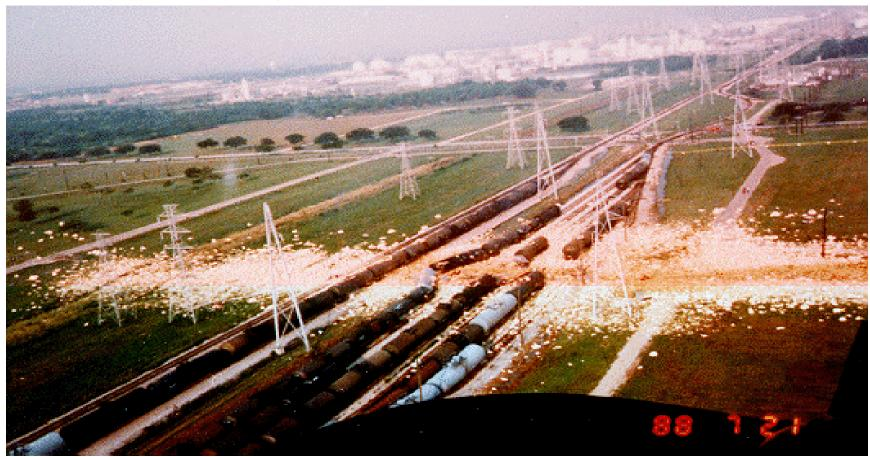
July 20, 1988: Tank-car of acid-washed MAA polymerized violently in Houston rail yard. MAA put in car had low inhibitor. Car was stainless, not normal lined car for this grade.  $H_2SO_4$  reacted with car walls.
