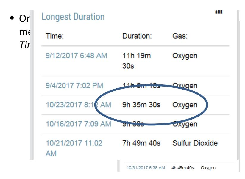
This is the actual datalog of the O2 reading showing no O2 in the environment—remember that the monitor was continuously in alarm on 10/23 for over 9 hours
