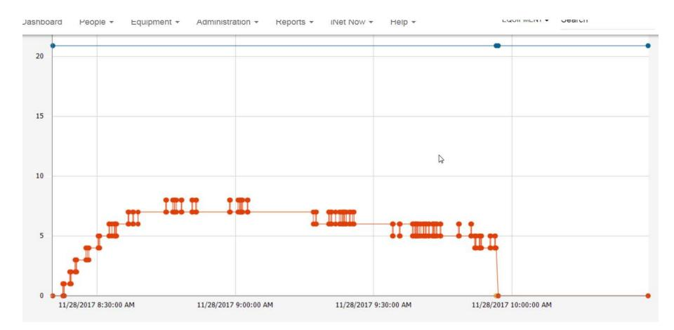
Typical curve of an actual CO exposure. Note the rapid recovery of the sensor. This exposure did result in a TWA alarm
